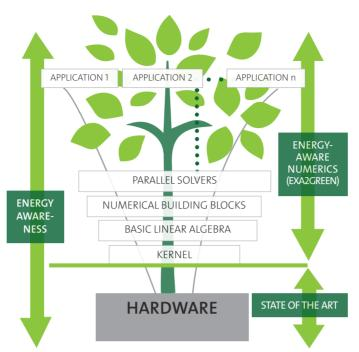
The concept of energy-aware numerics is a multi-level approach in which all layers from kernels, numerical building blocks to application level are designed by means of an optimized trade-off between energy consumption, performance and accuracy.
